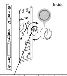
Note: Notch on cylinder must be in the 9 o' clock position when fully screwed into lock body.
