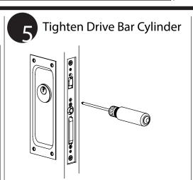
Tighten locking screw to engage notch on cylinder
