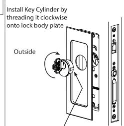
Key Cylinder notch must be at the 3 o'clock position when fully screwed in lock body.
