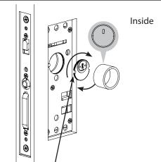
Note: Notch on cylinder must be in the 9 o' clock position when fully screwed into lock body.
